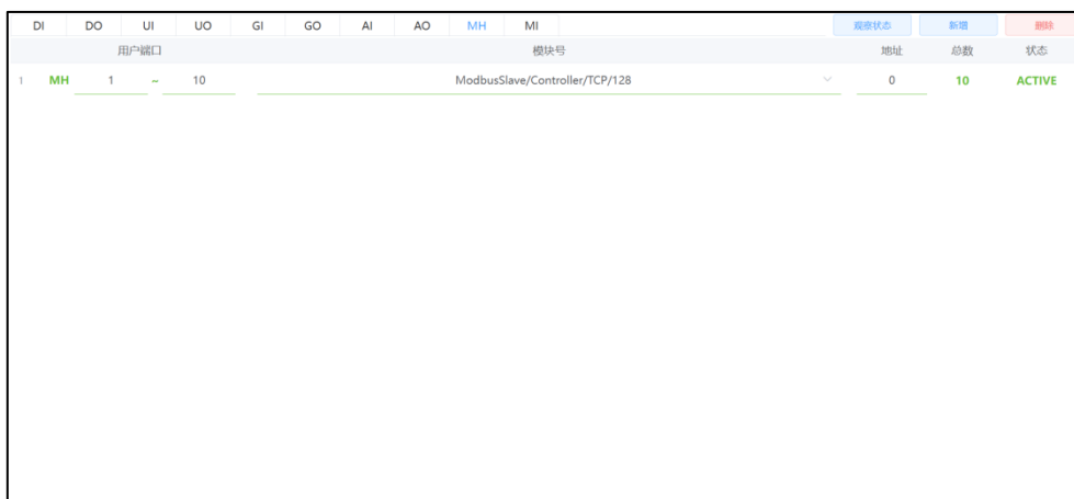
Fig. 6.2 Bus Register Signal Setting Screen
